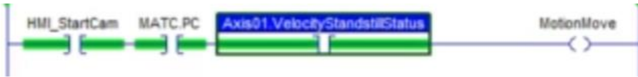
Figure 2 one possible cam start logic.
